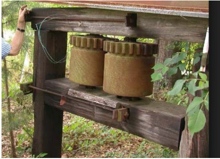
Sugar cane press similar to Bunea design
