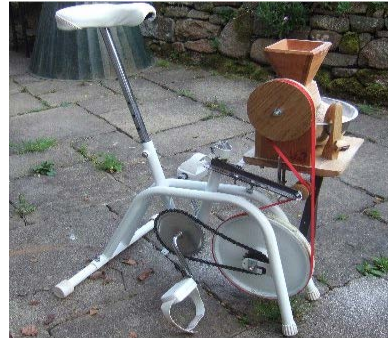
Multigrain grinder driven by a bicycle
