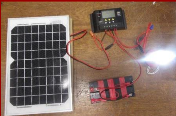
Figure 2: Prototype of the off-grid solar panel system (L) and the as-built system in Kampung Palipikan, Sabah, Malaysian Borneo (R).
