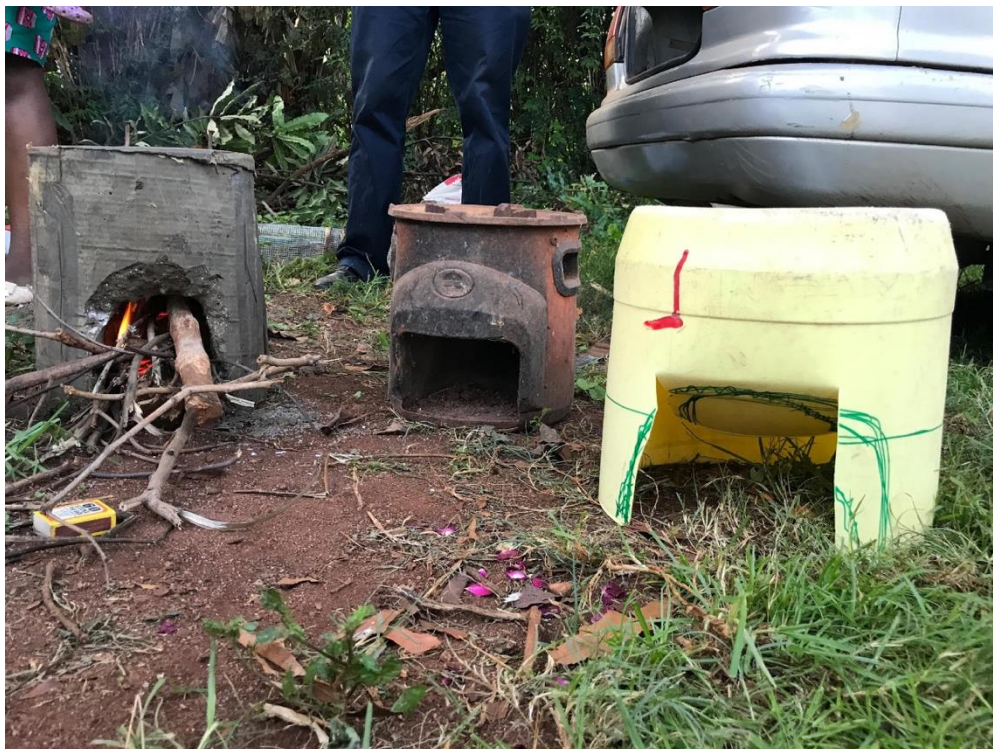
From left to right. Portable Jiko Stove prototype in the testing, commercial Jiko Stove, mould for the portable Jiko Stove.
