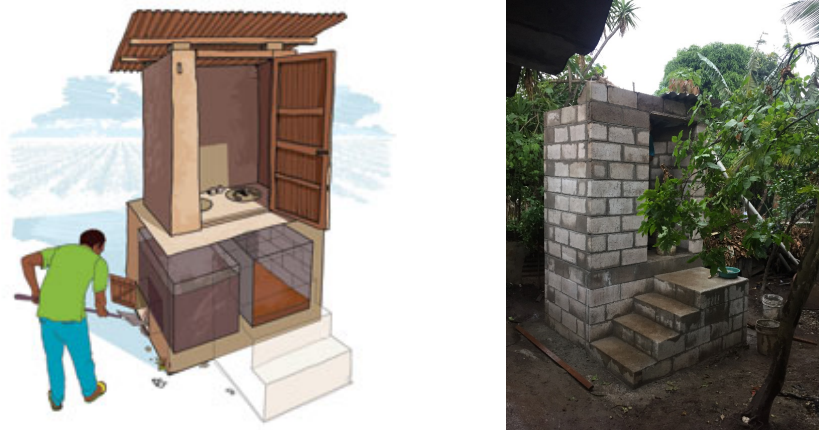
Figure 5: Schematic of composting latrine (left). Photo of composting latrine constructed (right).
